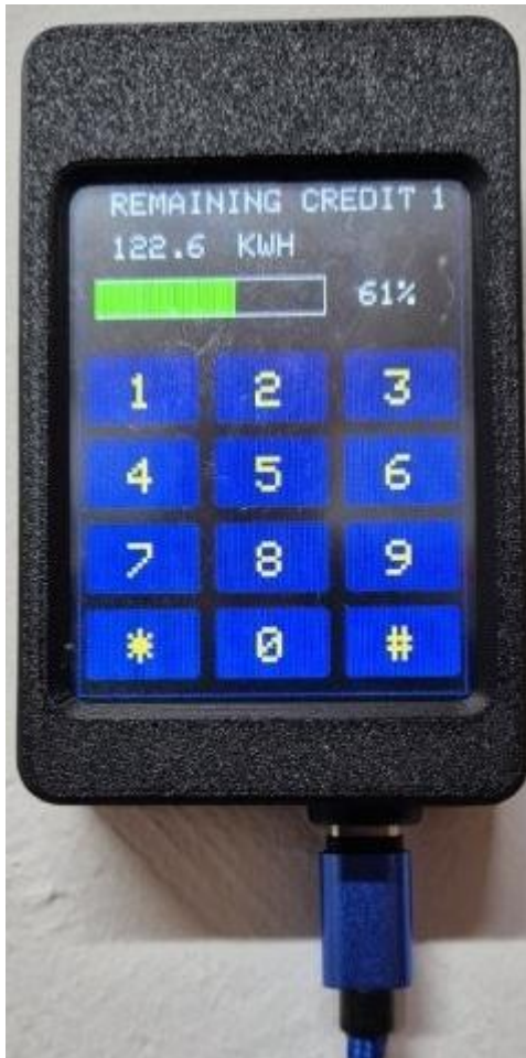
![[Photo 1: Front view of keypad showing display, keypad layout, and normal operation with remaining credit display]]
