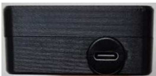
![[Photo 2: Bottom view showing USB-C connector for power]]
